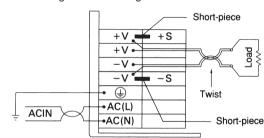
(2)When using remote sensing function
