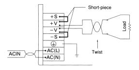
(2)When using remote sensing function
